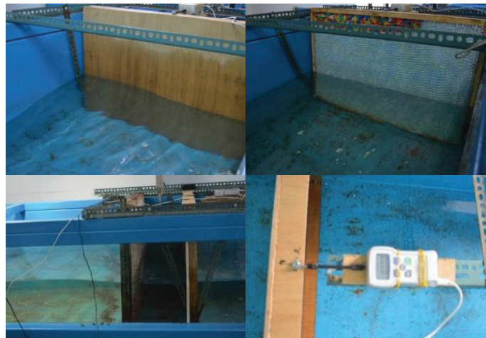
Fig.2 Photograph of experimental setup and impact force measurement.
